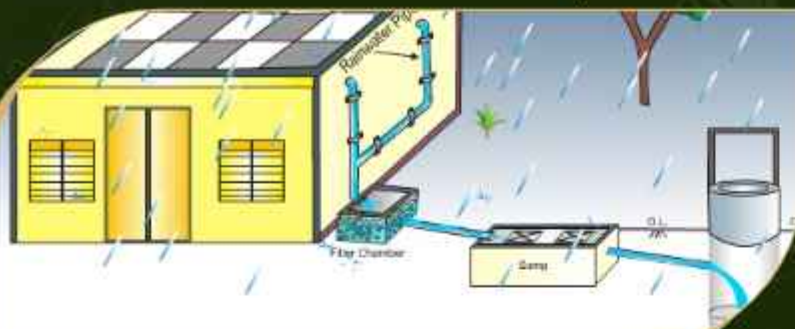
Rain Water Harvesting System
